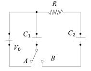
**Solution:** Since the switch was at A for a long time, the capacitor  $C_1$  will have voltage  $V_0$  across it. The energy required to raise the voltage of  $C_1$  to this voltage is
