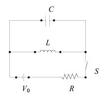
**Solution:** When the switch S is opened, we have only an LC oscillator. The current through the inductor at t = 0 will be  $I_0 = V_0/R$ , because that was what was going through it before the switch was opened. We can then find the current through the inductor as a function of time for t > 0. It will be
