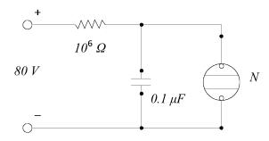
**Solution:** The time at which the first flash occurs will tell us the period of the flashing, which can then give us the frequency. The voltage across the capacitor is given by
