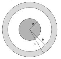
(a) First we need to calculate the electric field inside the insulating cylinder (r < a). Using Gauss's Law on an imaginary cylindrical surface of length l and radius r, and using the dummy variable s, we find
