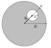
(a) This problem requires the application of superposition. First, suppose that the sphere is completely solid. Then, we can use Gauss's law to find the electric field at any distance r from its centre. First, take the origin of the coordinate system to be at the centre of the sphere. Then we have
