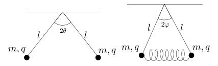
(a) When the spring is introduced, the system will reach an equilibrium, where for an appropriate choice of k, the distance between the two masses is  $2l \sin \varphi$ . This means that the spring will be stretched by  $l \sin \varphi$  from its initial length. Let's consider the forces on the left particle. If the tension in the rod is T, the force equilibrium in the y direction is
